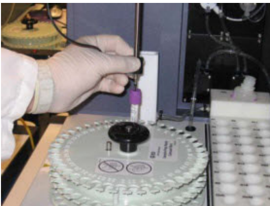
Figure 7-15 Pulling the probe arm down into the empty tube
