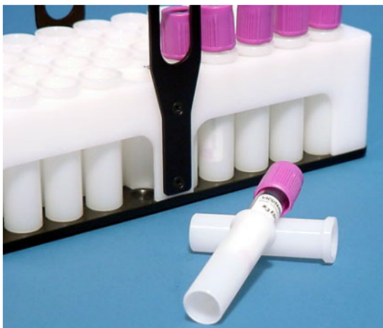
Figure 2-2 White tube adapters for primary tube rack
