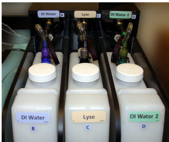
Figure 3-5 Color-coded labels and fluid connectors on tanks
