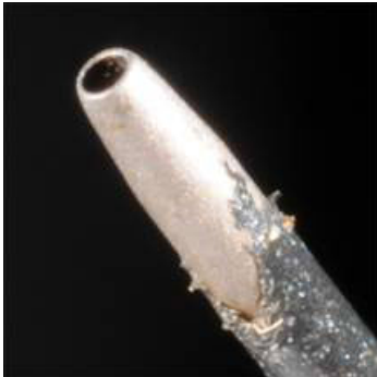
Figure 7-8 Probe with badly worn coating
