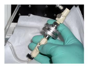
Hold the filter assembly with the printed face up and twist the locking rings in opposite directions to open the assembly.
