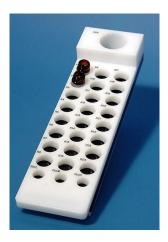
Each reagent rack position is numbered. The reagent vials sit in the rack at a slight angle to maximize reagent usage.
