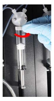
**Tip** If you twist the syringe a quarter turn in the opposite direction, and then in the direction shown, it will help seat the threads.
