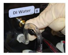
**9** Fill all the bulk fluid tanks in the fluidics tower.
