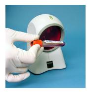
The white indicator light on top will flash once and a beep will sound when a barcode has been successfully scanned.
