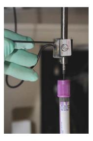
3 Slide the insulation block off of the Z-rack. The probe is attached to the fluidics tubing inside the Z-rack.
