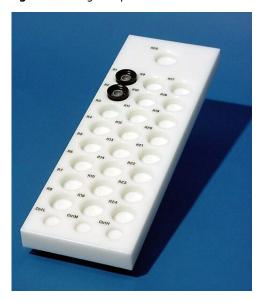
The reagent cap holder is numbered to match the reagent rack to keep caps organized and contaminant-free while you are preparing samples. Store the reagent cap holder on the benchtop during sample preparation.
