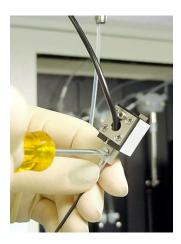
4 Attach the tubing to the new probe through the insulation block, and press firmly until it stops (Figure 6-11 and Figure 6-12).
