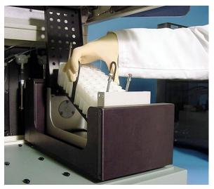
The primary tube rack should slip easily into the cage. If it does not, try turning it around. The numbers 1–40 should appear right-side up when the rack is in the correct position.
