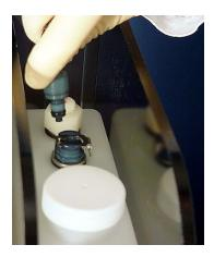
Firmly push the sensor connectors into the ports on the fluidics tower.
