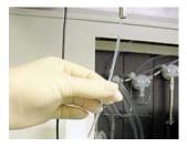
If the tubing is not accessible from below, you can push the tubing down from the top of the Z-rack.
