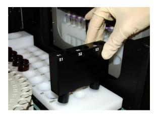
You can place up to three uncapped primary tubes in positions S1, S2, and S3. They must contain at least 150  $\mu L$  of sample plus the volume of sample to be dispensed. Keep the tubes capped until you are ready to start the run. Mix the tubes and then remove the caps just before you begin the run.
