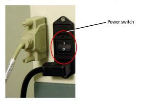
Leave sufficient room on the side of the instrument so you can easily access the power switch, which is located directly above the power cord.
