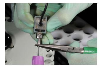
Keep the probe inside of the tube at all times. Dispose of the entire tube and probe into a sharps container.
