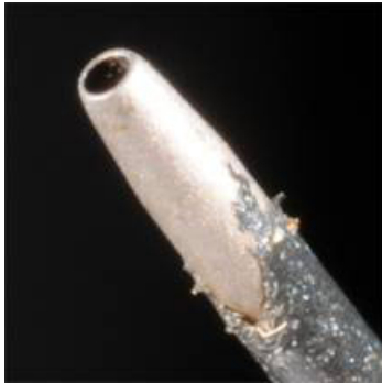
Figure 7-8 Probe with badly worn coating
