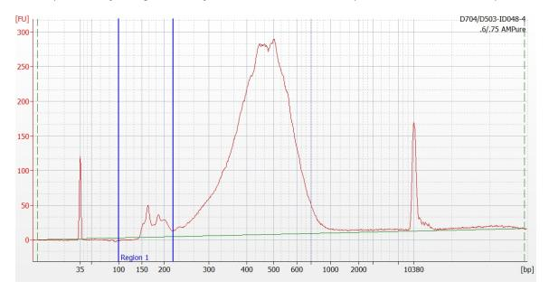
B. Sample Bioanalyzer high-sensitivity DNA trace for an index PCR product with an observable peak <270 bp
