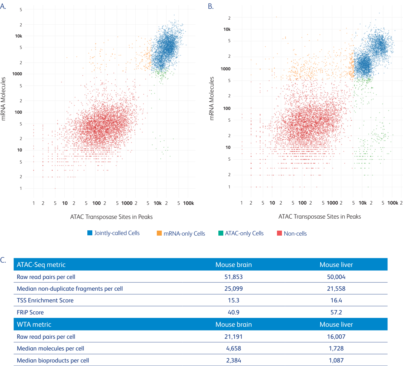
Figure 7. BD Rhapsody™ Single-Cell ATAC-Seq Assay performance with tissue samples. A) Scatter plot from a multiomic BD Rhapsody™ ATAC-Seq experiment with nuclei isolated from frozen mouse brain tissues isolated using the S2 Genomics Singulator™ Platform and prepared following the BD Rhapsody™ Nuclei Isolation Protocol, shows the FRiP score, a measure of specificity, against the number of transposase sites in peaks, a measure of sensitivity at roughly 50,000 mean raw read pairs per putative cell. B) The same plots from a BD Rhapsody™ ATAC-Seq Assay experiment with nuclei isolated from frozen mouse liver tissues isolated and prepared following the BD Rhapsody™ Nuclei Isolation Protocol and sequenced to the same depth. The divide in the jointly called cell populations (in blue) represent two different hepatocytes and endothelial cells from the liver tissue, that exhibit different levels of gene expression and open chromatin accessibility. C) ATAC-Seq and WTA metrics from the same experiments.
