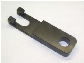
Figure 6-27 Deflection plate removal tool
