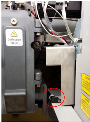
Figure 5-8 Mini-USB cable in retracted (1) and extended (2) positions
