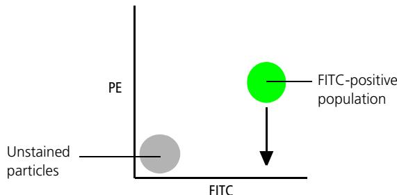
Using the Compensation tab of the Cytometer window in BD FACSDiva™ software, you can adjust the PE-%FITC spectral overlap value. Compensation is optimal when the positive and negative FITC populations have the same medians in the PE parameter statistics.
