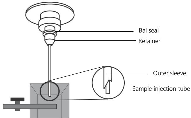
Work carefully. The outer sleeve can fall off as you loosen the retainer.
