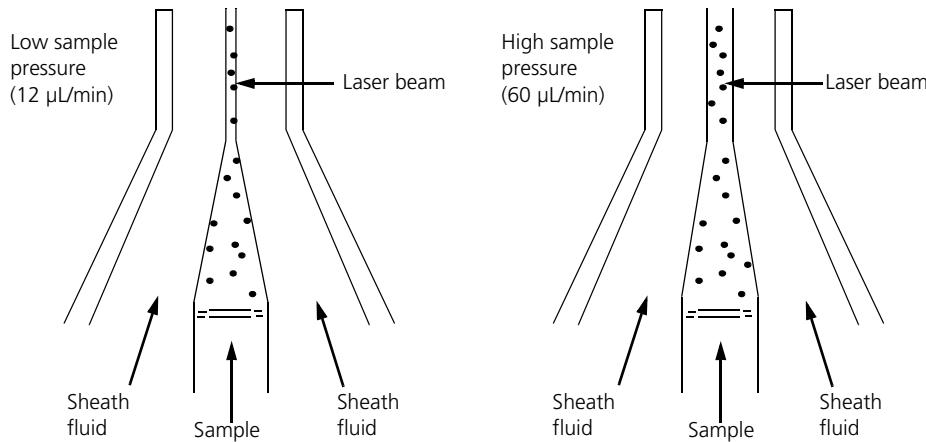
The objective in flow cytometric analysis is to have at most one cell or particle moving through a laser beam at a given time. The difference in pressure between the sample stream and sheath fluid stream can be used to vary the diameter of the sample core.
