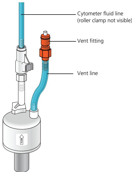
2. If bubbles are visible, gently tap the filter body with your fingers to dislodge the bubbles and force them to the top.
