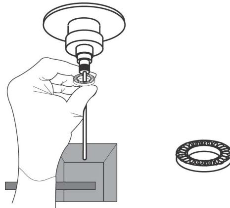
3. Install the new Bal seal spring-side up.
