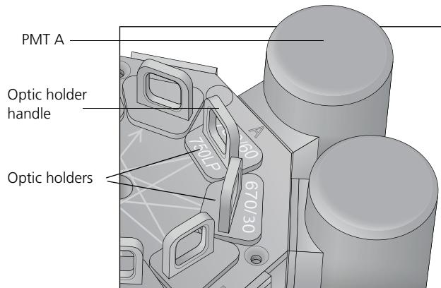
The filters steer progressively shorter wavelengths of light to the next detector in the array as indicated by the lines and arrows on the top of the polygon.
