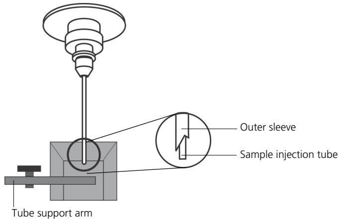
**Sample injection tube.** Stainless steel tube that carries sample from the sample tube to the flow cell. This tube is covered with an outer sleeve that serves as part of the droplet containment system.
