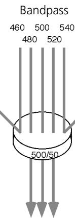
The performance of an optical BP filter depends on the optical transmission. Sample transmission curves are shown in the following figure. A filter with a narrower (steeper) transmission curve generally yields higher performance. The transmission specifications depend on the construction of the filter.
