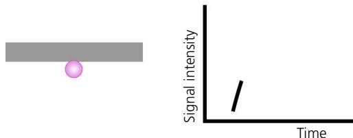
2. The pulse reaches a maximum intensity or height when the particle reaches the middle of the beam, where the beam and signal intensity are the brightest. The peak intensity, or height of the pulse, is measured at this point.
