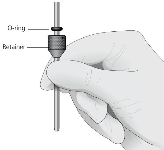
3. Invert the outer droplet sleeve and allow the O-ring to fall onto the benchtop.
