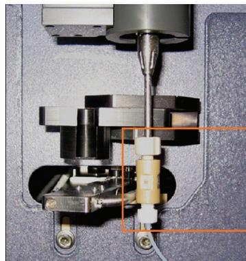
Verify that the sample coupler is properly installed and not leaking.
