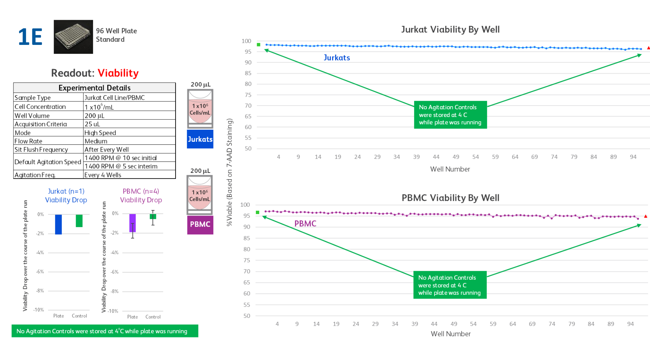
Figure 1E. Impact of Default Agitation Settings on Viability: Using a well volume of 200 µL, and default agitation settings (1400 RPM, every 4 th well for 5 seconds), the viability of both Jurkats (upper plot) and PBMC (lower plot) were measured for each of the 96 wells over the course of a plate acquisition. Cell viability was measured by 7-AAD staining. As a reference, a no agitation control was measured - aliquot of Jurkats or PBMC that was stored at 4°C during plate acquisition. The viability of the no agitation control was tested before and after running the plate.
