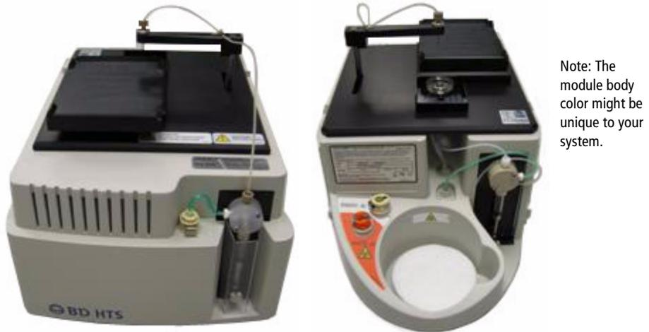
**NOTE** The main HTS module shown is the same for all BD LSR products. The BD LSRFortessa analyzer has an extra protective cover that mounts to the original BD LSR II HTS cover.
