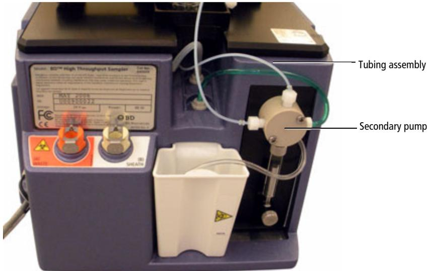
The tubing nuts are normally finger tight. If it is difficult to unscrew a tubing nut, use a 5/16 wrench to loosen it.
