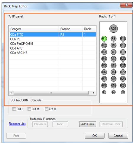
Select a reagent, then click a position on the rack map to assign it. Repeat until all reagents have been assigned to a position on the map.
