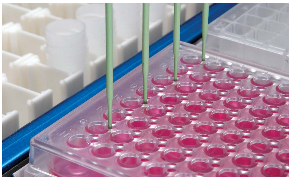
Media exchange through access ports using TECAN Genesis® RSP 150 liquid handler.
