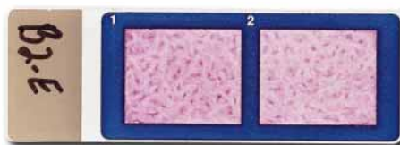
Photograph of primary bovine aortic endothelial cells grown on BD Falcon CultureSlides and stained with crystal violet. The blue hydrophobic grid defines the cell culture area. A white writing patch provides clear sample identification. Well location numbers etched in the grid are clearly visible.
