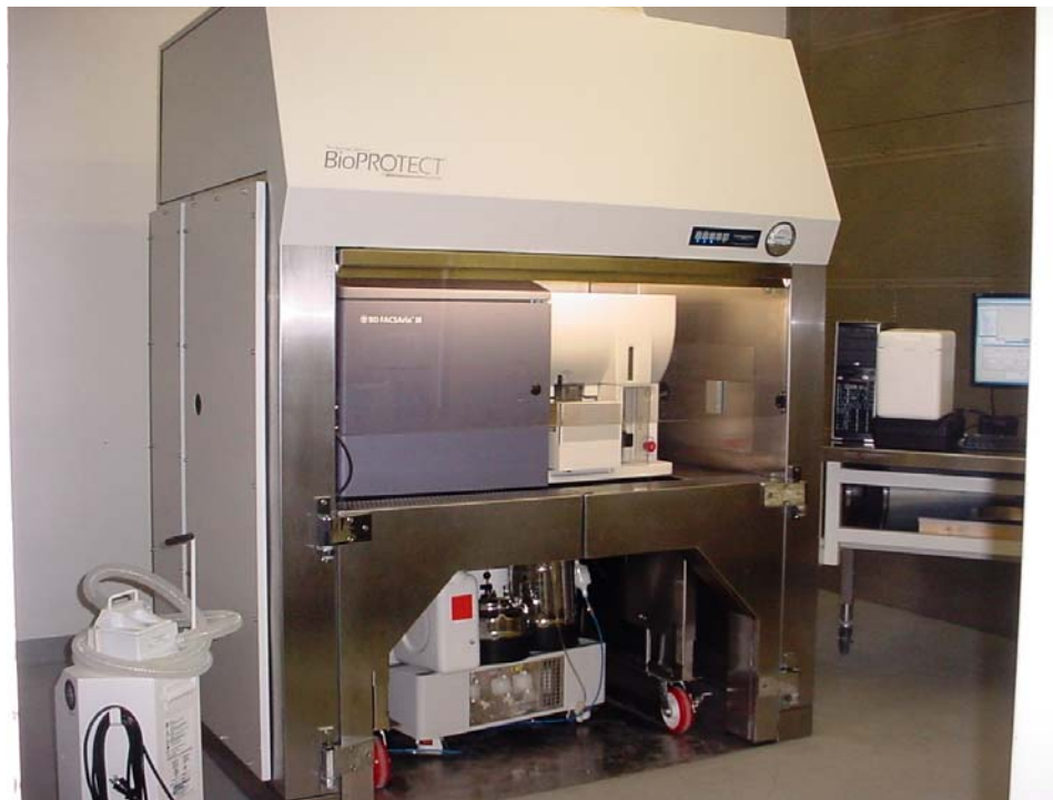
BioPROTECT IV with installed BD FACS Aria cell sorter plus Fluidics Cart
