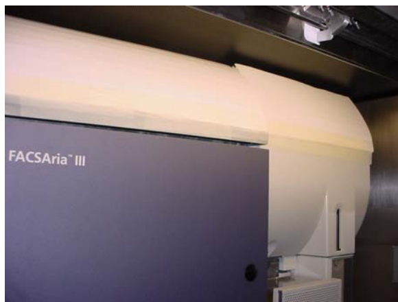
Air Deflectors on top of FACS Aria III
