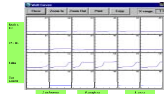
Fig. 6 Determination of efficacy in 6 hours. Using a slight modification of the general test protocol, the disinfectant efficacy on borosilicate glass cylinders was determined in a 24-well sensor tray. Controls were detected in 3 to 5 hours, whereas no fluorescence increase was observed in test (ready-to-use and 1:50 dilution) and negative control (sterile cylinders) wells. Manual observation of fluorescence intensity showed a strong signal in positive wells, as compared with weak background fluorescence in negative wells.
