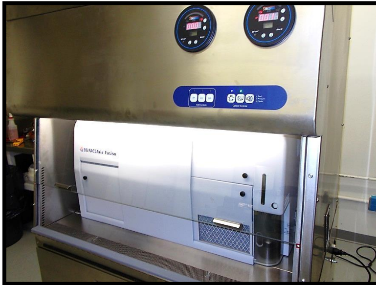
Figure 2 BD FACSAria Fusion inside safety cabinet
