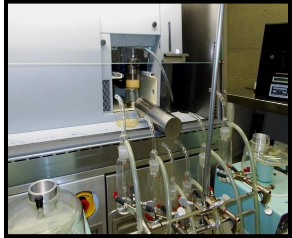
Figures 10, 11 Personnel Protection Microbiological Test at the Sort Chamber
