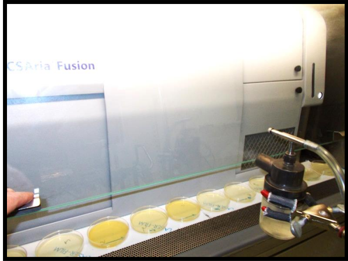
Figure 15 Example of Dynamic Product Protection test while closing the viewscreen
