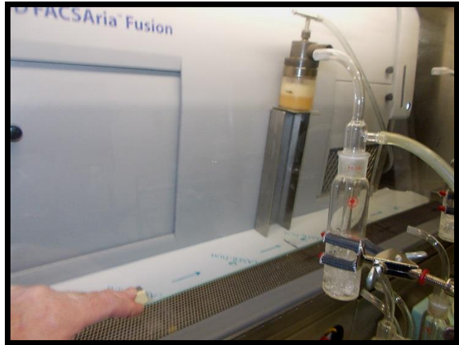
Figure 14 Example of Dynamic Personnel Protection test while closing the cabinet viewscreen
