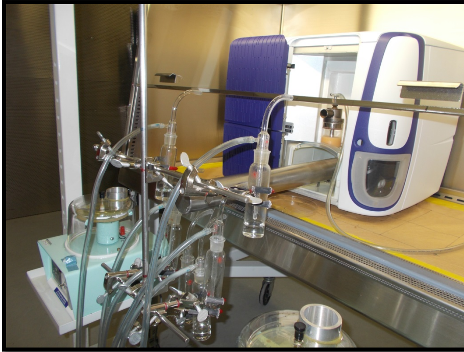
Figure 6 Personnel Protection Testing with Nebulizer inside the sort chamber
