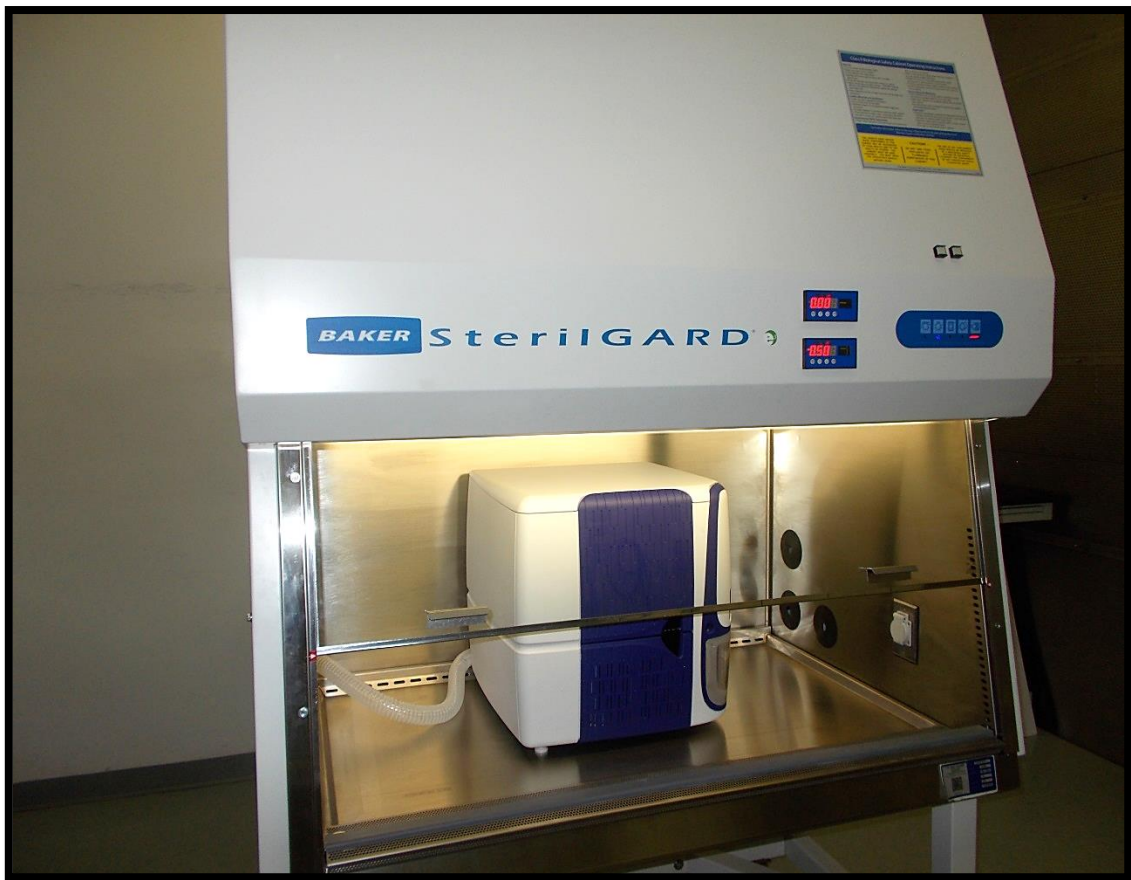
Figure 1 BD FACSMelody Cell Sorter inside the modified SterilGard BioSafety Cabinet
